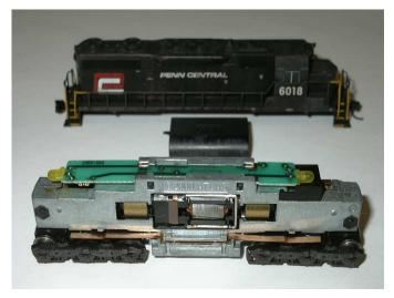
The fuel tank and shell are easily removed.
