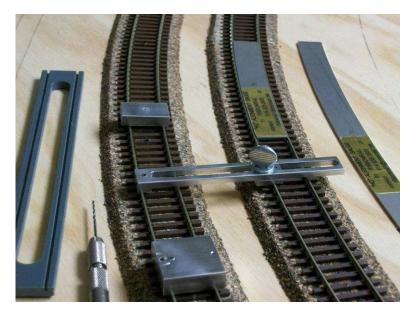
Clockwise from left: MLR straight alignment tool, flex track drill jig, Ribbonrail curved track alignment gauges, adjustable curved/straight track parallel tool, power feed hole drill jig, pin vise with drill bit.
