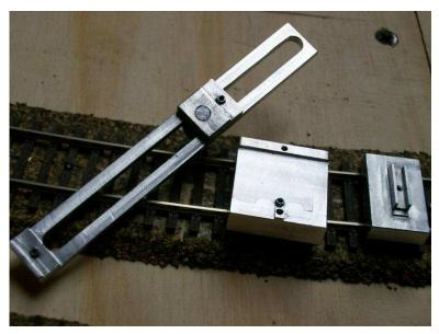
Left to right: adjustable curved/straight track parallel tool, power feed hole drill jig, flex track drill jig.
