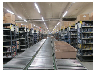
Main belt at Walthers. Start on the left and move toward the viewer, then continue up the right belt. Completed orders are put moved to the middle belt and head to the far end for packing and shipping.
