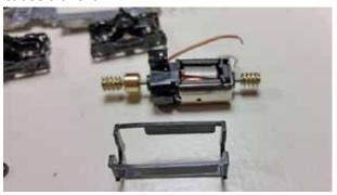
Remove the motor from the cradle, and remove the ineffectual seeming electrical tape insulation.
