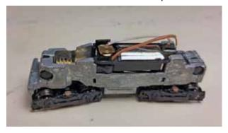
The mechanism with the non-DCC light board removed.
