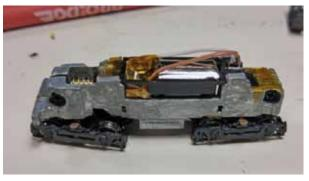
The solder pads on my decoders were too thick, so I had to give them a gentle, but firm, squeeze in some pliers to make them thin enough to fit into the slots in the mechanism. Finally, slide the decoder in and push the motor leads into the connectors.
