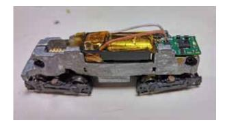
There are some important precautions that must be taken when installing DCC decoders in Micro-Trains's SW1500s. The MTL SW1500s were welcome additions to the N Scale world. Despite their too-wide hoods, they fill a huge gap in available diesels. Even better: despite using the DCC un-friendly Life-Like designed SW1200 mechanisms, they've been upgraded to be able to accept a "plug and play" decoder.
