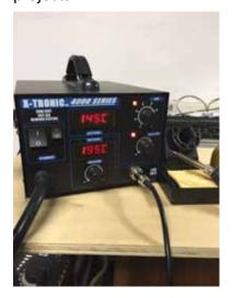
The unit is able to make the temperature changes quickly because the heating element is not a metal core as you find in most other irons. The heating element is a ceramic rod inclusive of a heating element, temperature sensor and ground surrounded by a metal tube, which attaches to a changeable tip. The changeable tip fits over the ceramic core.
