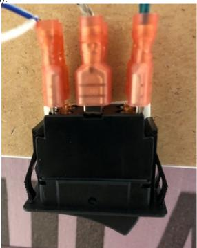
The DPDT switch is a simple device with lots of possibilities. The pair of terminals down the center of the switch is the main bus. The pair of wires on the left are from a Kato DC power pack, and the pair on the right is connected to an NCE Power Cab system. With a simple flip of the switch, the layout can be easily changed from DC to DCC and back without any rewiring. I secured the switch to the benchwork with double-sided tape.
