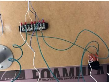
. Pardon the jumble. Although it looks somewhat chaotic, it works, and no soldering is required. The main bus between the DPDT switch (black box at bottom right) and the rest of the layout consists of two green 16 awg wires screwed into the terminal strip. The other side of the terminal strip is all of the feeder wires from the track, with the polarities separated between the two sides of the strip.
