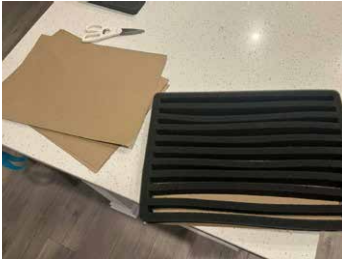
Without backing and bottom strips, thin foam rows cannot maintain shape.
